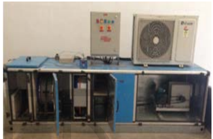
Figure: 1. Photographic View of Solid Desiccant assisted Hybrid Air-Conditioning System setup
